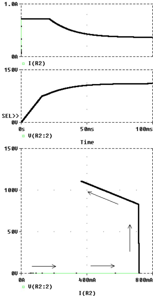
Figure 7. Startup simulation with a 40-W ONU load,  $R_W = 80\Omega$ ,  $L_W = 2.4mH$ , and  $C_{ONU} = 150\mu F$ . Lower figure is the state-space trajectory with inductor current on the horizontal axis, and capacitor voltage on the vertical axis.
