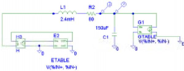
Figure 6. Pspice circuit for state plane simulations.
